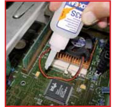
Cyanacrylate adhesives are for the instant and structural bonding of rubber, metals, ceramic, leather and a variety of plastics. Best results can be obtained with joint gaps of less than 0.1mm up to 0.2mm for special grades. The service temperature range is between -50°C and +80°C, although new high-temperature resistant formulations are available for use up to 200°C. For porous surfaces or for vertical application a gel grade is available.
