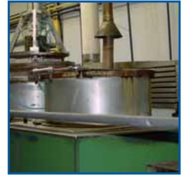
Low viscosity methacrylate resins for sealing metal micro porosity by vacuum impregnation of castings and sintered metal parts for automotive, pneumatic and hydraulic components. LOXEAL impregnation products meet the standards MIL-STD276, MIL-I-17563B and most automotive companies specifications.
