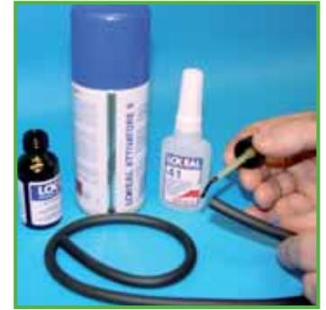
The activators are specially designed products to speed up the cure of Anaerobic Adhesives. Typical conditions of use are low temperatures, large gaps, inactive or passive surfaces.
