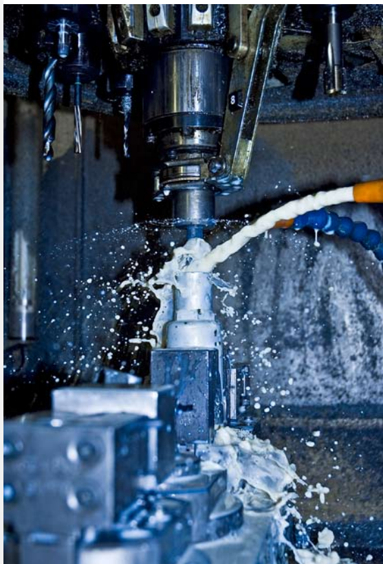
From our own production. Above the machine work on a pneumatic pump 5:1 on a machining centre.
