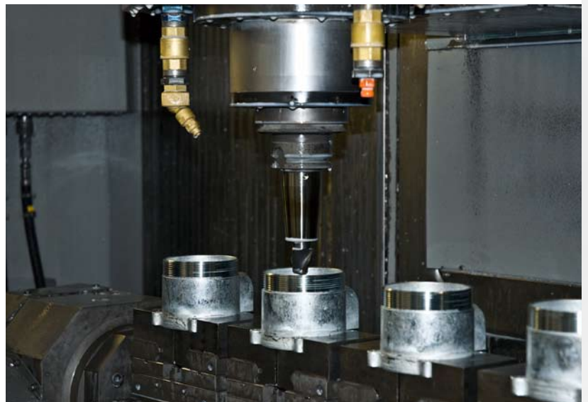
From our own production. Above the machine work on a pneumatic pump 5:1 on a machining centre.
